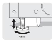
Stationary Front Roller with Leveling Screw
